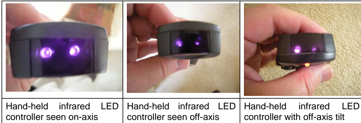
Figure 11. To illustrate the use of digital camera imaging to capture invisible infrared LED emitters, these images of a video remote controller were taken on-axis and slightly off-axis in two planes. Knowing the dimensions of the window, the actual source size can be quickly determined. A metric rule is sometimes placed adjacent to the source for more direct calibration.
