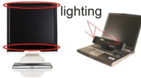
Figure 4. Remote VOG gaze tracking systems 3
