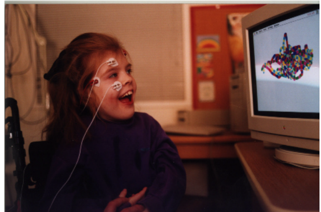
Figure 2. Eye painting with EagleEyes, electrodes measure the EOG [Gips and Olivieri 1993].
